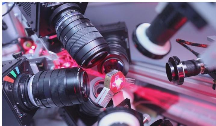
**Fig2.** The setup designed and constructed by Sergey Farisenkov for high-speed recording of the free flight of microinsects under infrared LED and laser illumination using four synchronized cameras. Photo from the archive of the Department of Entomology, Faculty of Biology, Lomonosov Moscow State University
