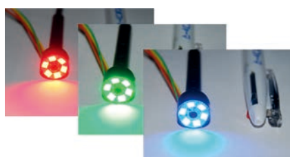
Microcirculation imaging device with LEDs and a small camera
